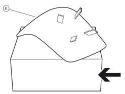
Please use one of the foam blocks to support and protect the concrete seat while placing the feet
